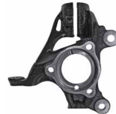
Light weight competences: this steering knuckle in Bionic design is more than 32% lighter than the standard design.
